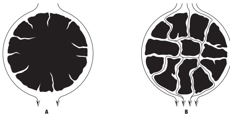
FIGURE 5.16 Transport of biomolecules through chromatographic media. A Conventional support particles. B POROS particles for perfusion chromatography.
