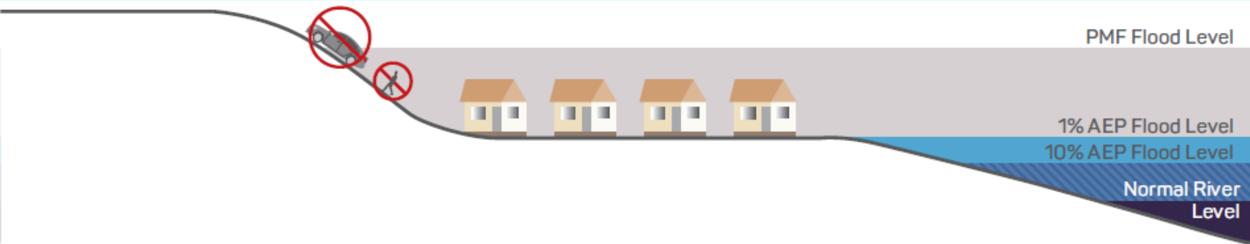
Figure 8: Example of area that is flood affected, isolated by floodwaters, and has impassable terrain and is fully submerged in the PMF. Category FIS.
