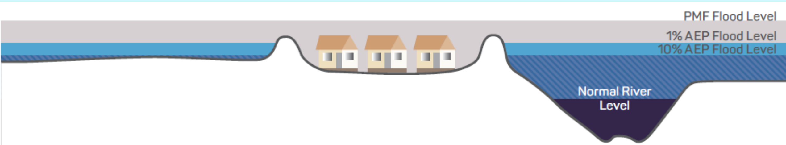
Figure 7: Example of area protected from the river by a levee designed for the 1% AEP event. In larger floods, including the PMF, the levee will overtop and fully submerge the entire area. access to the Area will be lost before overtopping. Category (FIS).
