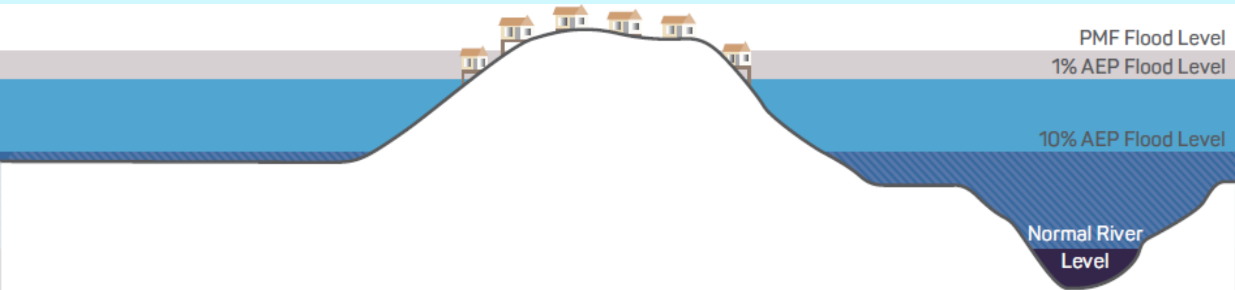
Figure 2: Example of area that is flood affected, isolated by floodwaters, but has some elevated area above the PMF. Category FIE.
