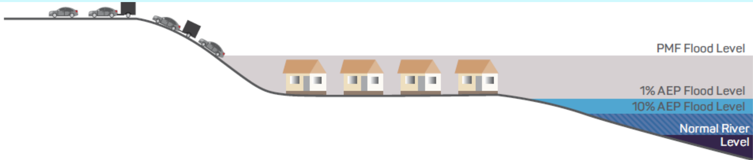
Figure 4: Example of area that is flood affected and has rising road access to the road network beyond the PMF. Category FER.
