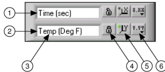
Figure 7.13: 1. X-axis, 2. Y-axis, 3. Scale Labels, 4. Scale Lock Button, 5. Autoscale Button, 6. Scale Format Button
