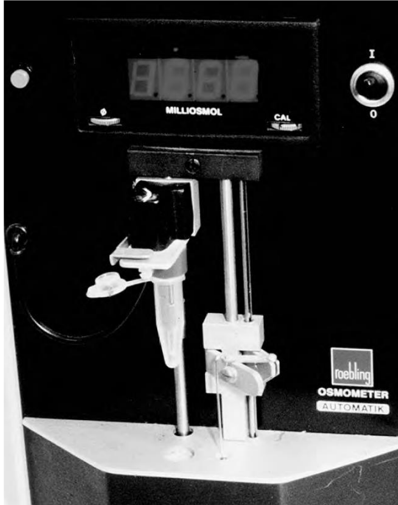
Fig. 9.1. Osmometer. Roebing osmometer (Camlab) showing front panel, sample tube, and sample port. This model accepts samples of 50 \mu L.
