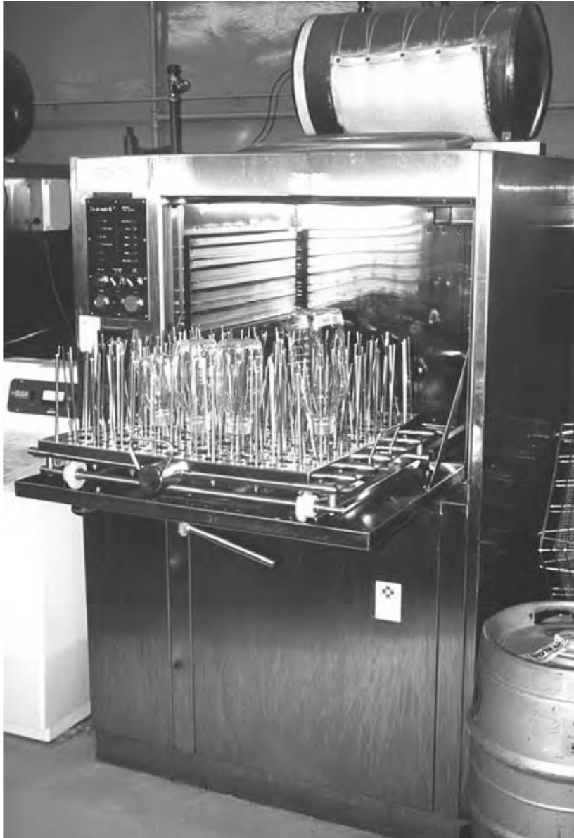
Fig. 5.21. Glassware Washing Machine. Glassware is placed on individual jets, which ensures thorough washing and rinsing (Betterbuilt).
