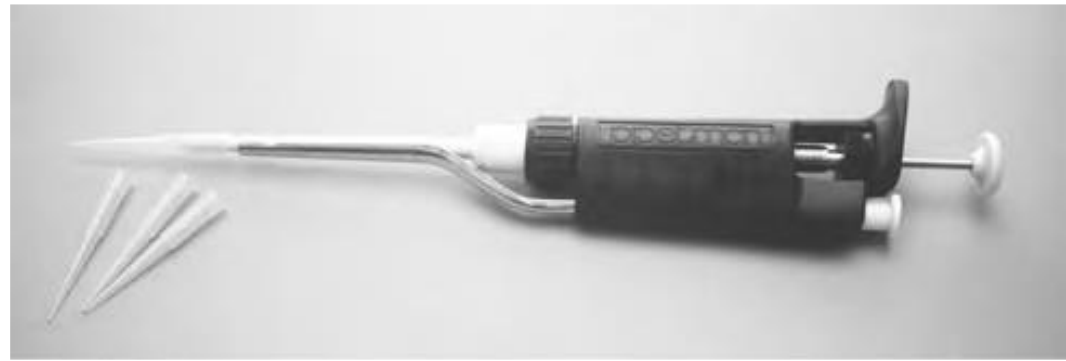
Pipettor. Variable-volume pipetting device. Also available in fixed volume. The pipettor is not itself sterilized but is used with sterilized plastic tips.
