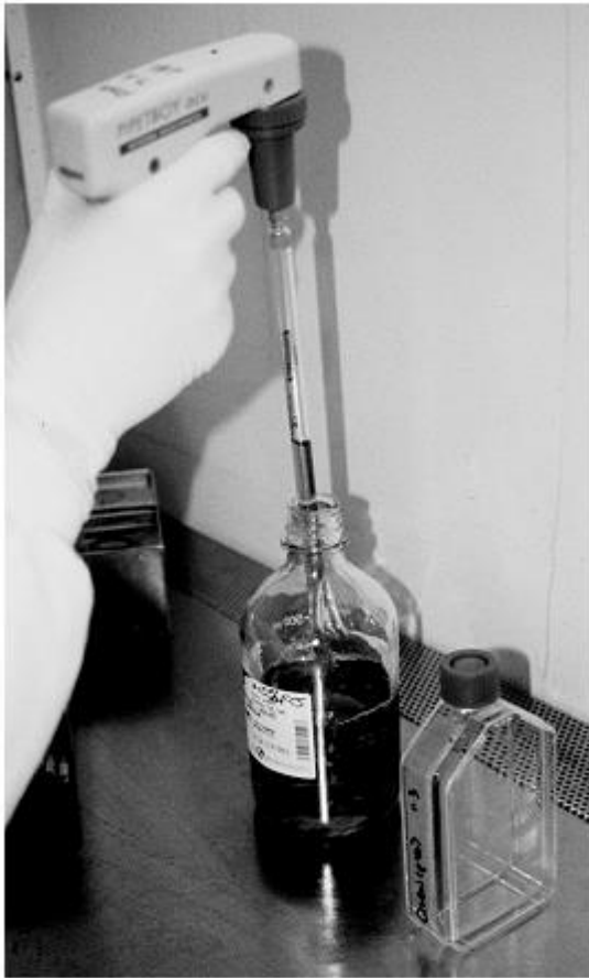
Pipetting Aid. Motorized pipetting device for use with conventional graduated pipettes.
